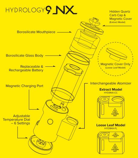
The Hydrology9 NX ships with either the Extract Atomizer or Loose Leaf Heating Chamber. Both the atomizer and heating chamber work with all NX units and can be swapped out at any time.
