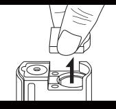
Remove the atomizer or heating chamber air path seal. You can clean the air path seal with a cotton swab, isopropyl alcohol, or water.
